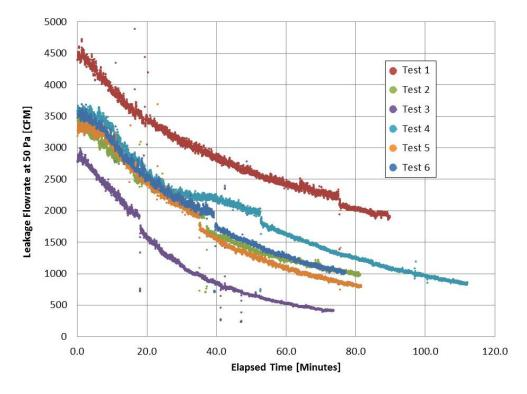
Figure 12. Sealing profiles for each of the sealing demonstrations performed
