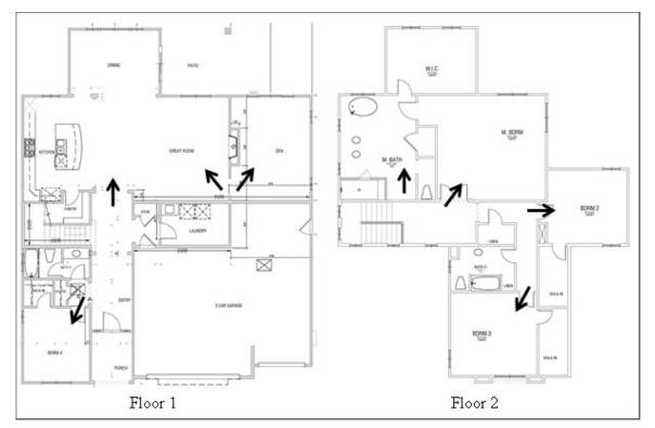
Figure 6. Diagram showing nozzles placement for one of the aerosol envelope sealing installations
