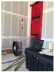
Figure 9. Blower door and aerosol injection hoses installed
