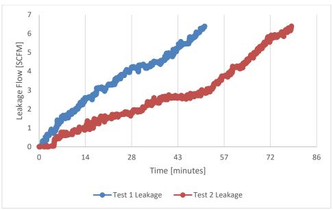
Figure 37: Leakage flow increase over time for ultimate failure test
