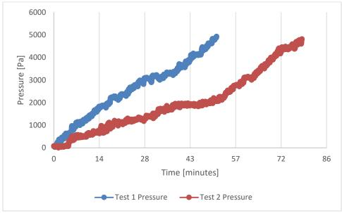
Figure 36: Pressure increase over time for ultimate failure test
