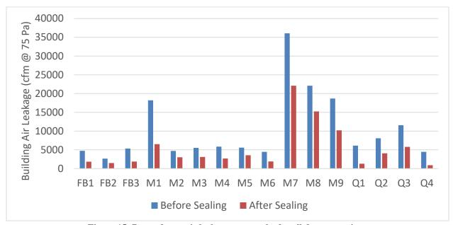
Figure 15: Pre and post air leakage test results for all demonstrations
