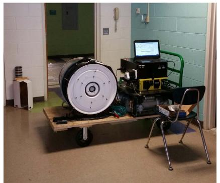
Figure 14: Photo of aerosol sealing equipment setup
