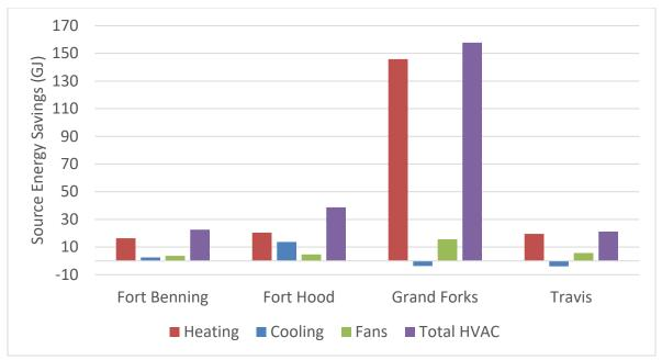
Figure 44: Modeled source energy savings for heating, cooling, and fan equipment due to air sealing
