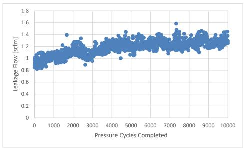
Figure 39: Leakage rates over 10,000 cycles of 800 Pa
