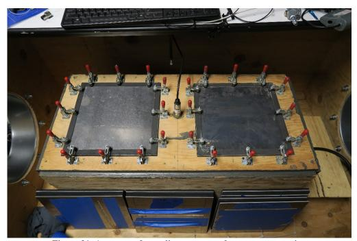
Figure 31: Apparatus for cyclic pressure and temperature testing
