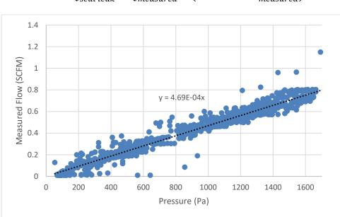
$$Q_{seal\ leak} = Q_{measured} - (0.000469 * P_{measured})$$
