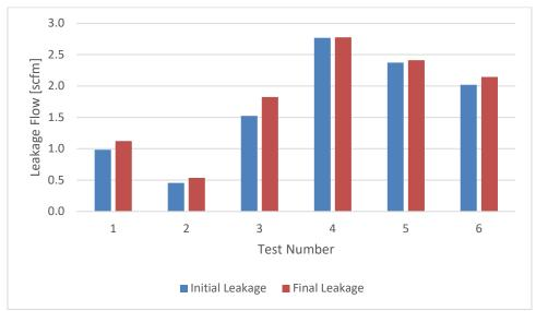
Figure 38: Change in leakage after 1,000 cycles of 800 Pa (note: Test 3 experienced a significant overpressurization resulting in higher percent change)
